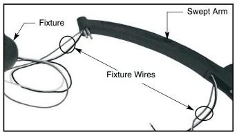
4. Install fixture to swept arm. Pull wire through swept arm and out arm access opening. Push wire into pole and out the top of the slipfitter.
