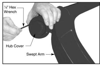
6. Install hub cover and secure with screws.
