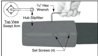
1. Slide hub slipfitter over tenon. <a href="Important! Orient slipfitter mounting holes in direction of Swept Arm assembly and tighten">Important! Orient slipfitter mounting holes in direction of Swept Arm assembly and tighten (4) set screws using a %6" hex wrench. (See "top view" above.)</a>
