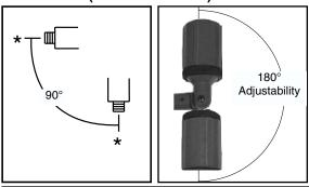
\*Note: Swivel stem must be installed with the mounting threads facing down-to-horizontal. Fixtures may not be installed with mounting threads facing upward unless shielded from rain or sprinklers.
