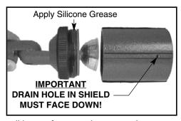
4. Install lamp of type and wattage shown on fixture label. NOTE: Add silicone grease to screw threads each time fixture is relamped.
