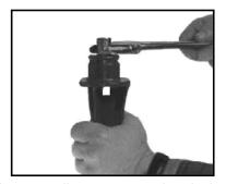
**1.** Tighten coupling onto mounting device. (See KIM Installation Instructions for Low Voltage Mounting Options, part no. 95488.)
