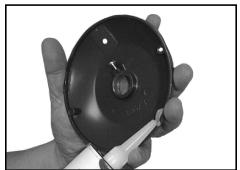
1. Attach mounting plate to J-box with screws provided. Apply clear silicone to inside of wall canopy to ensure water tightness.
