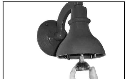
5. Install lamp of type & wattage as shown on fixture label and chart. Reinstall lens and lens frame. (Step 5 not required on L.E.D. version, for L.E.D. fixture skip to step 6).
