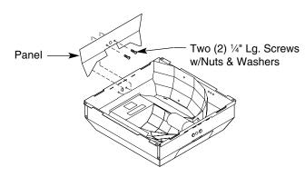
3. Install panel opposite socket using ½" lg. screws with nuts and washers.
