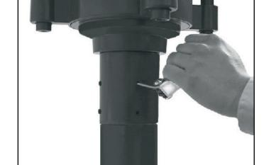
3. Tighten (4) set screws securely using a <sup>3</sup>/<sub>16</sub>" hex wrench. Remove one screw, drill recess in tenon or pole for screw point, and replace set screw.
