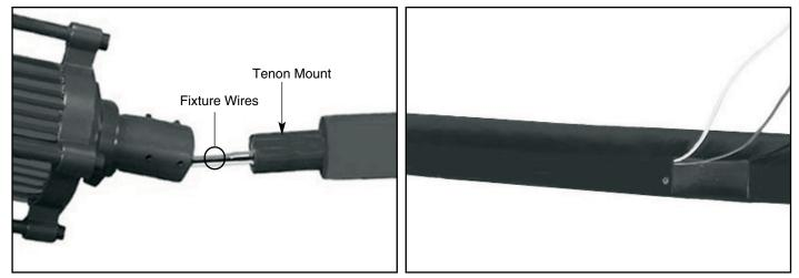
1. Lay pole on padded support to protect finish. Feed supplied pole wiring through tenon opening, down the pole and out hand hole.
