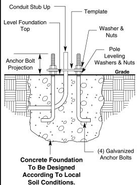
**Note:** Pole base <u>must</u> have full contact with foundation by grouting. Provide a channel through the grout for drainage from the pole interior.
