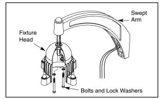
3. Install bolts and lock washers through fixture head as shown. Pull wires through arm and out arm access cover. **IMPORTANT: Keep wire tight** when attaching fixture to arm to avoid pinching wires.
