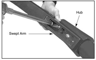
2. Install swept arm hub with bolts, tighten to 20 ft.lbs.
