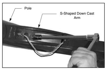
4. Attach down cast arm to pole. Tighten to 20 ft.-lbs.
