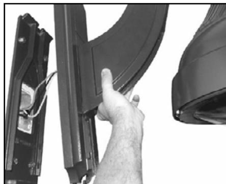
5. Attach wall mount cover plate with arm and fixture head attached, to wall plate with two (2) 5/16"-18 x 1 1/4" socket head cap screws. Connect fixture wires to supply wires observing polarity, i.e.; green-to-ground, white-to-common, and black-to-voltage. (See fixture installation instructions.)
