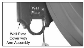
Attach wall plate cover assembly to wall plate. Secure with two (2) socket head cap screws. Connect fixture wires to supply wires observing polarity, i.e.; green-to- ground, white-to-common, and black-to-voltage.
