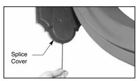
7. Attach splice cover using the 10-32 flat head stainless steel socket screw. Follow fixture installation instructions for fixture attachment.
