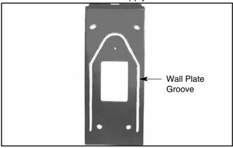
1. Remove wiring inspection cover from wall plate and wall mount cover plate. Adhere rope caulk in a continuous strip into the wall plate groove. Allow caulk to extend well above the wall plate surface to ensure a proper seal.
