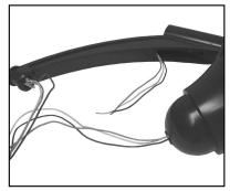
2. Pull wire through arm and out arm access cover.
