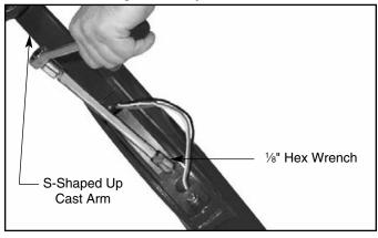
Attach up cast arm to pole with bolts, tighten to 20 ft.lbs. All mounting hardware is supplied by Kim Lighting.
