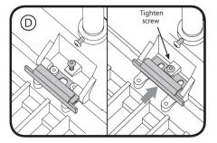
Swing luminaire closed and secure with the slide clip. Lock slide clip in place with screw.
