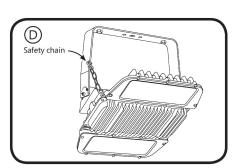
**NOTE:** Optional safety chains can be used in 3/8" holes in sides of bracket and in the mounting slots at the end of fixture.
