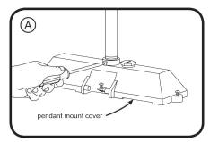
Attach pendant mount cover to 3/4" NPT conduit. Determine rotation of luminaire and lock orientation in place with provided set screw.
