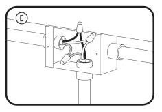
Connect the green (ground), black (line) and white (neutral) wires of the AC line to the similarly colored wires of the luminaire's lead wire using UL listed wire connectors. Close junction box.
