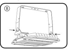
Lift fixture up and insert provided (2) 1/4" hex drive bolts through brackets, then install provided locknuts.
