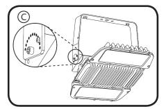
Determine rotation of fixture and lock orientation in place (both sides) with provided (2) 1/8" hex drive screws
