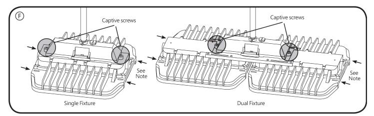
Secure pendant mount cover to luminaire by fully tightening the captive screws on the sides of the pendant mount box to the fixture. **NOTE:** Safety chains can be used in mounting slots at end of fixture.
