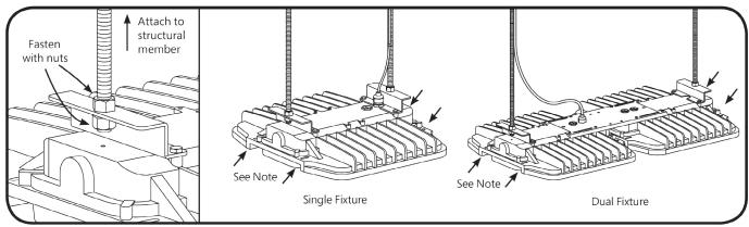
Secure two 1/2" threaded rods into structural members in ceiling. Place a nut on each threaded rod where fixture should hang. Slide rod mount brackets onto threaded rods and tighten second nut onto rods to secure fixture.
