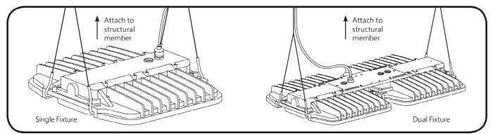
Hang two chains/cables from a structural member of the ceiling. Fixture must be supported independently of an outlet box. Loop chain/ cable through the mounting slots next to each fixture end. Chain/cable mounting locations must be in the slots at the ends of the fixture.
