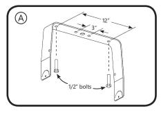
Mount U-bracket to a flat wall or ceiling surface using (2) 1/2" bolts. Use either the 3" or the 12" hole pattern.
