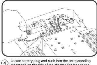
Locate battery plug and push into the corresponding receptacle on the side of the charger. Proceed to the Electrical Connections section to complete.
