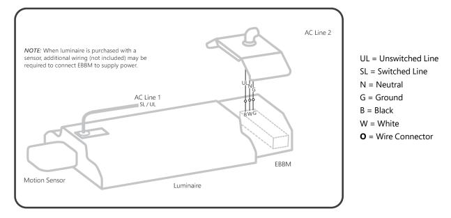
Switched Luminaire with EBBM & Motion Sensor with One Power Drop
