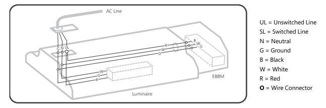
Luminaire with EBBM & Motion Sensor with Two Power Drops
