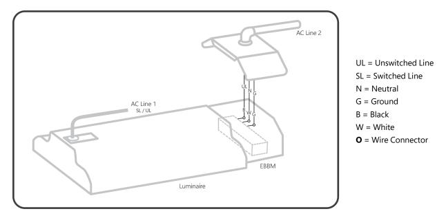
Switched Luminaire with EBBM with One Power Drop
