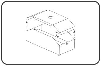
Loosen two screws to remove the top cover of the EBBM unit.
