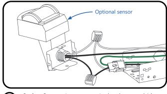
**Option:** Sensor – Insert sensor (ordered separately) into endcap knockout (provided in Continuous Run Kit) and wire to starter wire harness per sensor wiring instructions. Replace closed endcap with assembled piece.
