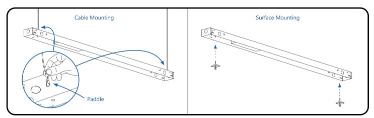
Hang fixture using either a pair of cables or mount directly to ceiling using appropriate hardware (not included).
