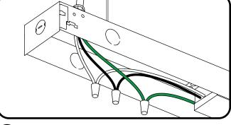
Install electrical fitting and feed the AC line wire through the fitting.
