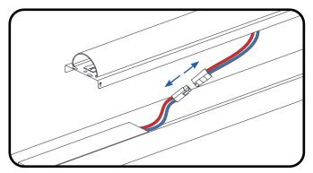
Remove cover and LED strip by disconnecting the quickconnectors to the driver.
