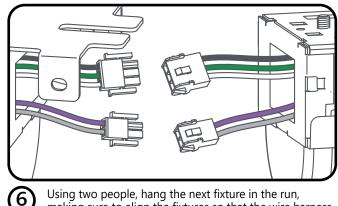
Using two people, hang the next fixture in the run, making sure to align the fixtures so that the wire harness quick connectors mate correctly.
