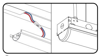
Reconnect similarly-colored wires from LED driver to LED strip. Reattach cover by sliding onto housing, reinserting screw. and replacing lens end cap.
