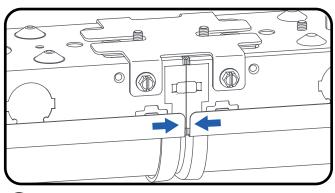
Push wire harness quick connectors into either fixture. Align bracket with adjacent fixture, push fixtures together, and drive one of the provided screws through the slot on each side of the bracket into the housing of the second fixture.
