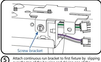
Attach continuous run bracket to first fixture by slipping over the top of the housing and driving one of the provided screws through the hole in each side of the bracket and into the housing.
