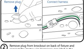
Remove plug from knockout on back of fixture and connect the starter wire harnesses provided in the Continuous Run Starter Kit.
