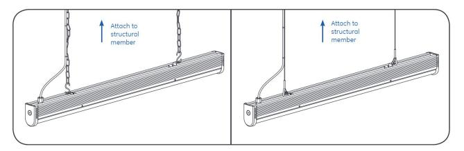
Hang two chains/cables from a structural member of the ceiling. Fixture must be supported independently of an outlet box. Loop chain/cable through the two mounting brackets.
