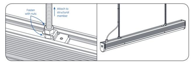
Secure two 1/2" threaded rods into structural members in ceiling. Place a nut on each threaded rod where the fixture should hang. Slide mounting brackets onto threaded rods and tighten second nut onto rods to secure the fixture.
