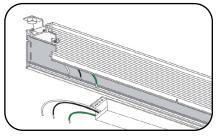
Remove driver from fixture and install new driver using same hardware.
