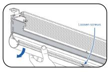
A Follow steps 3b through 3d of Surface Mounting to remove fixture cover.
