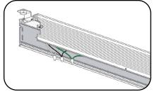
Disconnect driver from any existing fixture wiring, take note of connections.
