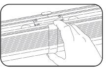
Snap on decorative lens cover (provided in Continuous Run Kit) over the seam between the fixtures.
