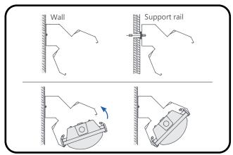
Mount the wrap-around brackets on the wall or support rail using appropriate hardware. After brackets are secured in place, install one side of the housing in the bracket, then rotate up and snap the other side of the housing into the bracket.
