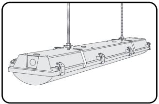
Mount the wrap-around brackets on the housing and then attach to the 3/8 inch rods using appropriate hardware.
