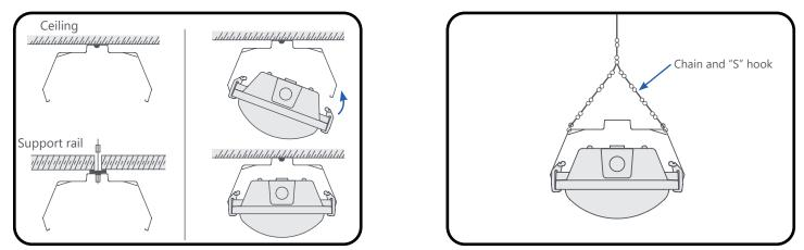
Mount the wrap-around brackets on the ceiling or support rail using appropriate hardware. After brackets are secured in place, install one side of the housing in the bracket, then rotate up and snap the other side of the housing into bracket. Chain and "S" hook (not included) can also be used to support the brackets.
