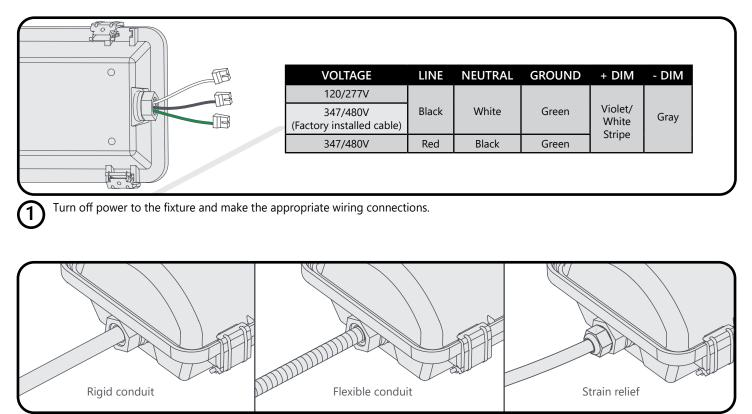
Connect a rigid conduit or flexible conduit or strain relief and feed the AC line wire through the fitting.
