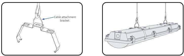
Snap the cable attachment bracket to the standard wrap-around brackets. Use appropriate cables to hang the fixture.
