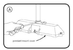
Attach pendant mount cover to 3/4" NPT conduit with at least 3 full threads of engagement. Determine rotation of luminaire and lock orientation in place with provided set screw.
