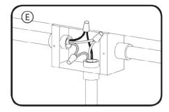
Connect the green (ground), black (line) and white (neutral) wires of the AC line to the similarly colored wires of the luminaire's lead wire using UL listed wire connectors.
