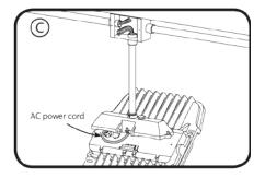
Feed the AC power lead wire through the conduit and into the junction box.
