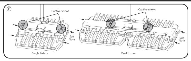
Secure pendant mount cover to luminaire by fully tightening the captive screws on the sides of the pendant mount box to the fixture. **NOTE:** Safety chains (installer provided) can be used in mounting slots at end of fixture.
