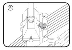
Lift luminaire up and hang on pendant mount cover using hinge piece.
