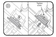
Swing luminaire closed ensuring power lead wires are not pinched and are fully enclosed in pendant mount cover.
