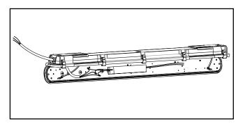
9. Secure lens to housing with lens latches.
