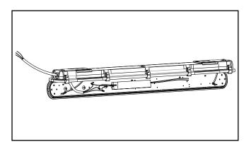
**8**. Reattach LED tray and lens to fixture by reversing step 4.
