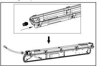
7 .Connect power to driver as shown in the figure. (the flexible cord supplied by others)
