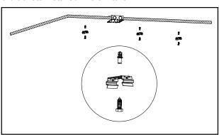
**3** . Secure mounting clips to housing recesses by firmly pressing them into place until both sides of the clip are secured.
