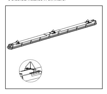
3. Hang fixture from customer supplied chain using V-brackets.
