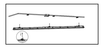
**4** .Release latches by pulling top of latch away from housing.
