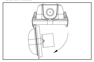
**2.**Fix mounting bracket on fixtures.
