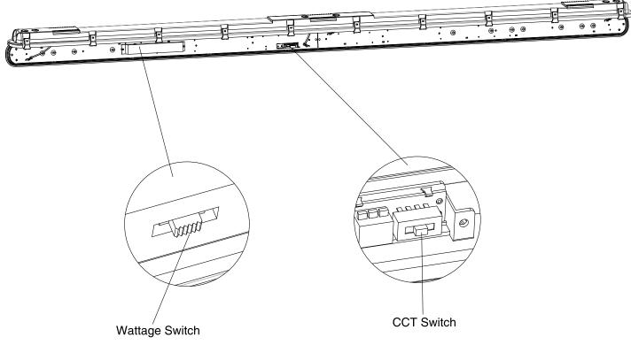
The end users may adjust the color temperature and lumen output respectively by the two DIP switch. Each DIP switch is accommodated with 3 options (left, middle and right), corresponding to 3 color temperatures and 3 powers respectively, which can perform the desired color temperature and lumen output combination.
