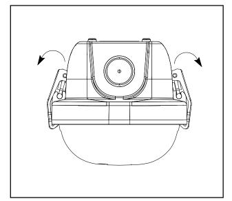
5. Without touching LED boards, detach LED tray and lens from fixture.
