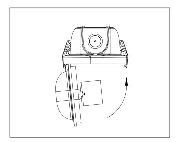
**9**. Secure lens to housing with lens latches.
