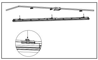
**5**. Without touching LED boards, detach LED tray and lens from fixture.
