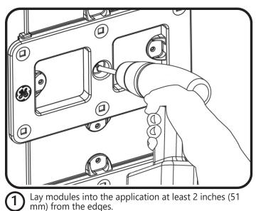
Fasten down each module with at least one screw in the center hole or two opposing sides.
