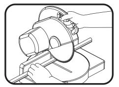
3 Cut the light guide to the required length using a hacksaw, chop saw (cross cut or veneer blade only), band saw, or other appropriate plastic cutting tool.
