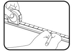
Mark the light guide at the required length, adding 0.5 in. (13mm) for every 16 in. (406mm) to account for shrinkage during the forming process.
