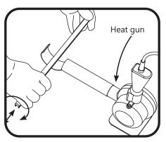
Move the section back and forth while rotating about the diameter until it is soft and pliable. Gently bend to the desired angle. It is recommended to use a heatdeflecting shield to distribute the heat evenly. Avoid localized overheating that may result in distortion or damage (i.e. bubbling) of the light guide.
