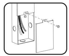
Mount LED driver and remove junction box cover. Carefully remove knockout for AC line input wires. Install appropriate electrical fittings in the knockout holes for wire protection.
