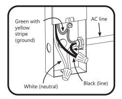
Connect the AC line to the black (line) and white (neutral) input wires of the LED driver using 18-14 AWG (0.82-2.08 mm²) twist-on wire connectors.
