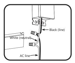
Connect the AC line to the black (line) and white (neutral) input wires of the LED driver using 18-14 AWG (0.82-2.08 mm²) UL approved wire connectors. Properly ground power supply in accordance with National Electric Code (NEC) Article 600.
