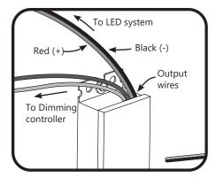
Connect the supply wire that is attached to your LED system to the red (+) and black (-) output wires of the LED driver as outlined in the "Electrical Connections" section of your LED system's Installation Instructions.
