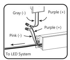
Connect the (+) purple and (-) pink wires of the LED Driver to the 0-10V dimming controller. Refer to the dimming controller installation instructions for specific connection information.
