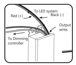
Connect the supply wire that is attached to your LED system to the red (+) and black (-) output wires of the LED driver as outlined in the "Electrical Connections" section of your LED system's Installation Instructions.
