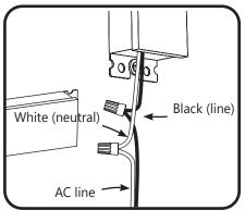
Connect the AC line to the black (line) and white (neutral) input wires of the LED driver using 18-14 AWG (0.82-2.08 mm2) UL approved wire connectors. Properly ground power supply in accordance with National Electric Code (NEC) Article 600.
