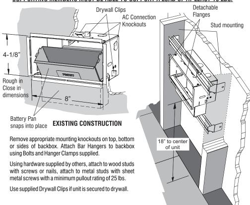
UNIT IS APPROVED FOR TYPE IC INSTALLATION.
