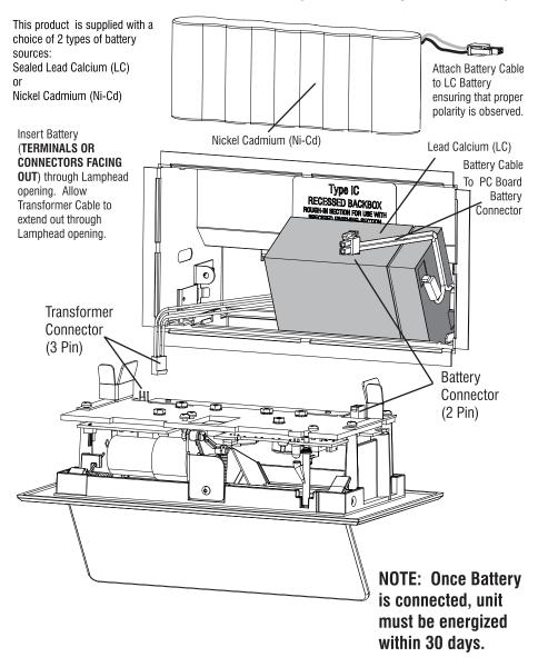
Connect 2 pin Battery Cable first, then 3 pin Transformer Cable to matching sockets on Printed Circuit Board. **BATTERY CABLE, WITH BATTERIES CONNECTED, MUST BE ATTACHED BEFORE AC POWER IS APPLIED.**
