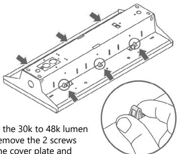
**Note:** For the 30k to 48k lumen version, remove the 2 screws holding the cover plate and slide to one side to remove it.
