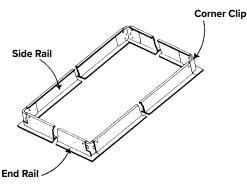
1. Cut ceiling opening to proper dimensions. Slip fit corner clips into side and end rails. No tools are required.
