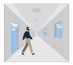
With sufficient daylight, the sensor keeps light OFF even if motion gets detected
