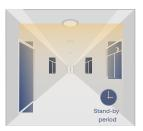
After holdtime, sensor dims light to standby dimming level for a standby period. If the standby period has been set to Os, sensor turns light OFF automatically after holdtime.
