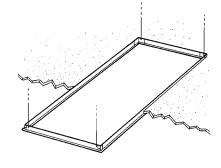
2a. Place Flange Kit in ceiling opening and wire each corner to ceiling structure. Pull up tight against ceiling.
