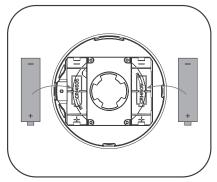
4) Install new batteries. then reverse previous steps to finish the battery replacement. (Only use CR14505 for WOS3 devices)
