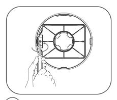
Remove device from ceiling by rotating counter clockwise. Then, unscrew the screw from battery housing cover
