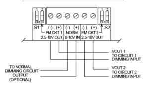
CAUTION: The sum of loads connected to Output Circuits 1 and 2 must not exceed unit rating in emergency mode.
