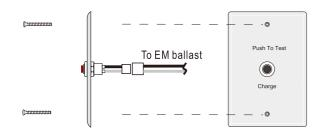
B. Install test switch on fixture surface.
