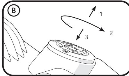
Lift, rotate, release, press to seat.
