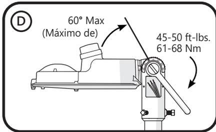
Adjust aim and tighten knuckle bolt.
