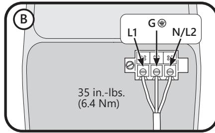
Secure wires in terminal block.
