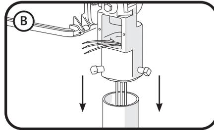
Thread wire and insert into knuckle base.
