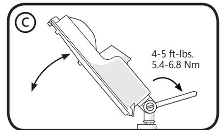
Adjust aim and tighten knuckle bolt.
