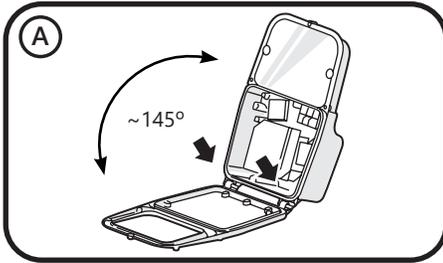
Hang door on hinge, rotate closed.
