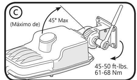
Adjust aim and tighten knuckle bolt.
