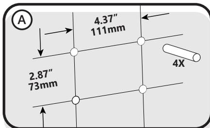
Drill mounting surface and insert 4 user-supplied anchors.
