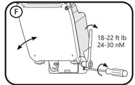
Orient luminaire, secure screw to hold position, tighten trunnion bolt.
