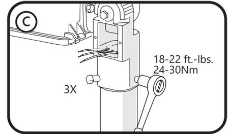
Tighten three (3) mounting bolts.
