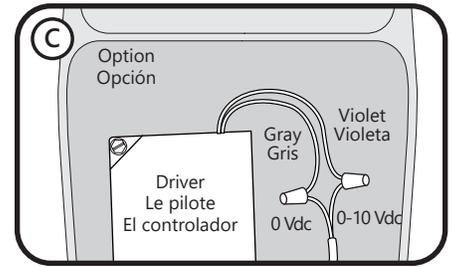
Connections for wired external dimming.
