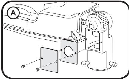
Remove wiring coverplate and gasket.
