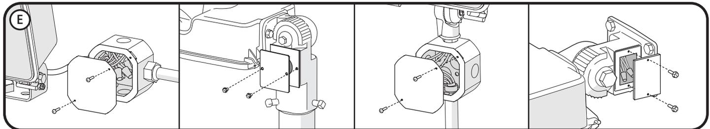
Insert wires and reinstall coverplate/gasket.
