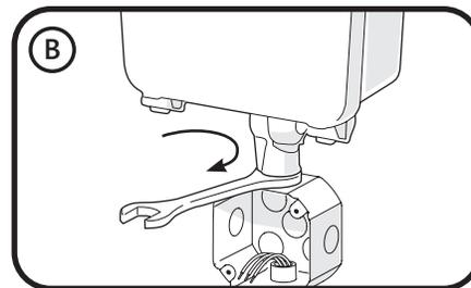
Securely mount the luminaire to junction box.
