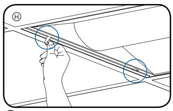
Secure swing door by locking latches found on the end of the assembled RVU Door.
