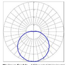
Maximum Candela = 1.159 Located At Horizontal Angle = 85, Verticle Angle = 2 #1 - Vertical Plane Through Horizontal Angles (85 - 265) (Through Max. Cd.)
