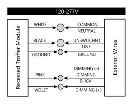
**NOTE:** Two sets of leads may be provided from the linear fixture labeled with black and white labels corresponding to "UV" and "WHITE" light circuits. These may be connected to the same or separate circuits depending on customer instruction. Dimming is not recommended on the UV circuit as it will reduce the disinfection effectiveness.
