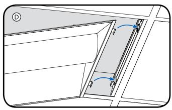
Install the RVU Fixture T-hinges into the RVU Mounting Bracket cutouts
