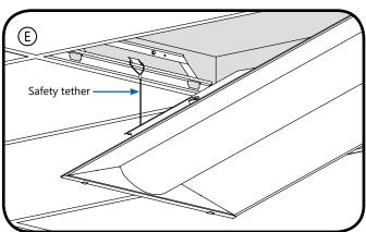
Secure RVU fixture to existing fluorescent fixture using provided safety tether. Ensure safety tether loop is secured around T-shaped tab in RVU Mounting Bracket.
