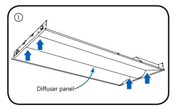
Please ensure diffuser is in place and secure, with no gaps between diffuser and housing. LEDs should not be visable. If diffuser is damaged or missing, do not install and please contact the manufacturer fro replacement.
