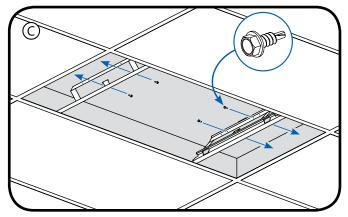
Install RVU Mounting Bracket to each end of the fixture by sliding RVU Mounting Brackets between the fixture and t-grid, ensuring the mounting bracket is centered in the fixture. Secure the RVU Mounting Brackets to the fixture using 4 of the provided #8 x 1/2" self-drilling screws.
