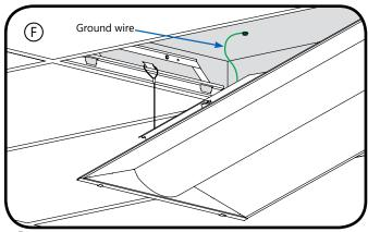
Install grounding wire using provided green ground screw (if existing hole is available) OR #8 x 1/2" self-drilling screw.
