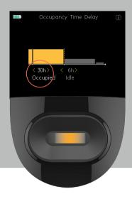
Use the CENTER button to enter editable features such as dimming levels.
