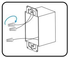
Terminate wires (previously connected to wall switch) with wire nuts.
