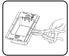
For proper installation into a dual gang junction box, the tabs between adjacent back housings must be removed.
