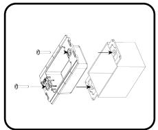
Install the back housing(s) of the wall dimmer(s) into the wall box.
