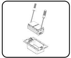
Use two standard screwdriver to remove the devices from the back housing
