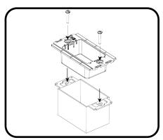
Insert the back housing piece into the junction box and secure with two screws. Reference Installation of Back Housing onto Junction Box instructions Steps 5 and 6 on Page 2 for more details.
