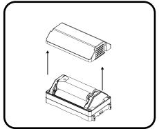
Separate the battery cover from the device. Pull the two plastic insulation strips out of the battery compartment. Put the battery cover back on the device.
