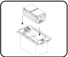
Install the main body of the device into the back housing.
