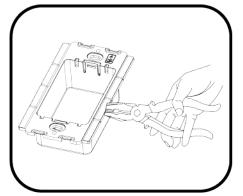
For proper installation into 5 a dual gang junction box, the tabs between adjacent back housings must be removed. Carefully observe the correct orientation (the UP arrow should be in the upper right corner on each back housing). After double checking the product orientation, break off the necessary tabs using pliers.
