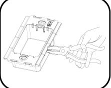
For proper installation into 5 a dual gang junction box, the tabs between adjacent back housings must be removed. Carefully observe the correct orientation (the UP arrow should be in the upper right corner on each back housing). After double checking the product orientation, break off the necessary tabs using pliers.
