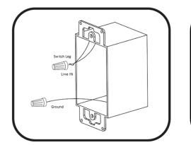
Terminate wires (previously connected to wall switch) with appropriate electrical connectors.
