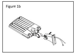
Step 2: Install fixture to pole or surface.
