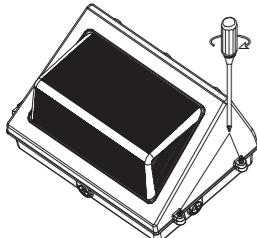
3. Use a screwdriver to remove the plug.
