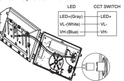
10. Switch power and CCT as part III, close the fixture and tighten down housing screws.
