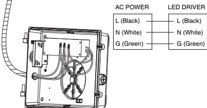
9. Install the cover of the fixture. Press the top of CCT switch and connect the wires back as diagram. Disconnect the photocell if no need.
