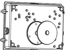
2. Open the fixture, press the top of cct switch, disconnect the wires (Blue,Gray,White), and remove the upper cover of the fixture.
