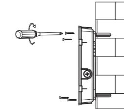
6. Use a screwdriver to remove the side plug and attach the EVA cotton pad to the mounting hole.
