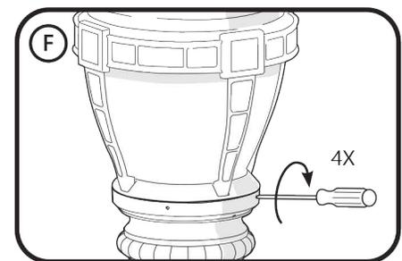
Tighten 4 screws to secure globe.
