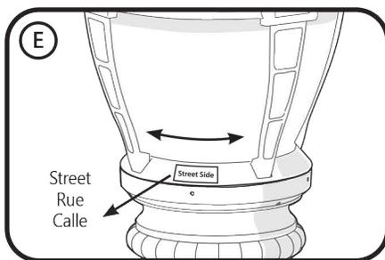
For correct PE orientation rotate globe with "StreetSide" label facing street.
