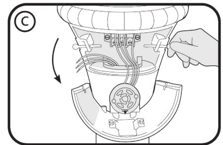
Loosen thumb screws to open access panel.
