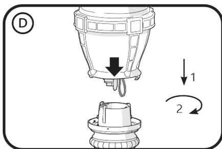
Lower globe into locking ring and rotate clockwise.
