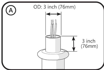
Place unit on 3-inch diameter x 3-inch long tenon (76mm x 76mm).
