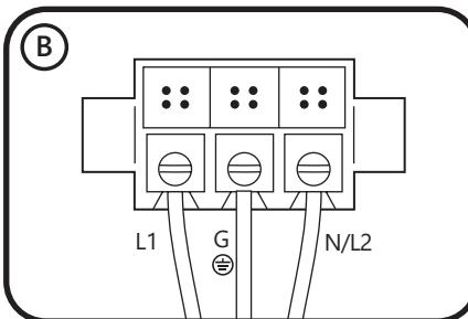
Connect leads. Torque screws per Table 1.
