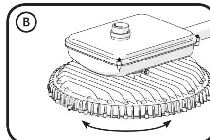
Rotate to desired orientation.
