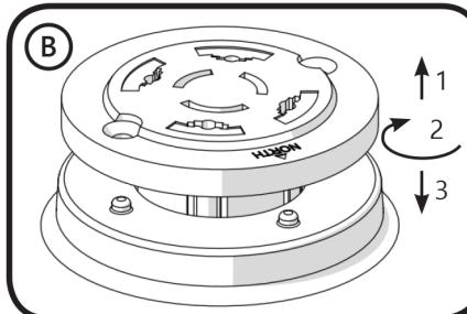
Lift, rotate, release, press to seat.
