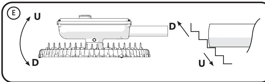
Luminaire may be tilted with respect to pipe. Shift steps to level fixture front-to-back.
