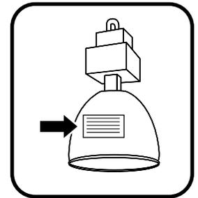
4. Close the fixture's junction box. Clean the area before applying the re-lamp caution label to a visible location on the fixture.
