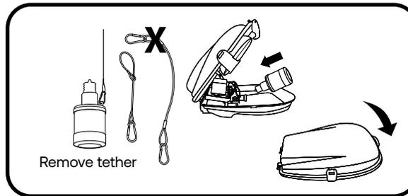
5B. Tether kit is optional for enclosed fixture applications. If using, please refer to the instruction for open fixture and check for no impact on secured closing of fixture door. If not using, please remove the tether kit. Install Current HID LED retrofit lamp into the socket and close the fixture.
