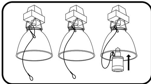
5A. Install Current HID LED retrofit lamp into the socket. Loop the wire of the tether around a load bearing building structure, then feed wire through loop at end of tether before using clip to attach to lamp. Minimize the length of the wire attached to the lamp. Zip tie extra loose wire if necessary.
