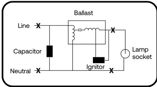
2. Open the fixture's junction box and bypass the HID ballast, ignitor (if there) and the capacitor (if there) by disconnecting the line and neutral wires and socket black and white wires in the locations with "CROSS" marks in the schematic diagram.
