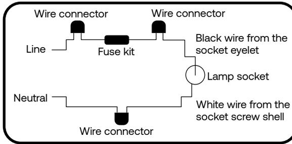
3. Connect the line to the black wire from the socket and the neutral to the white wire from the socket with UL listed wire connectors. The fuse kit in the package should be installed on the line as shown in the schematic diagram.
