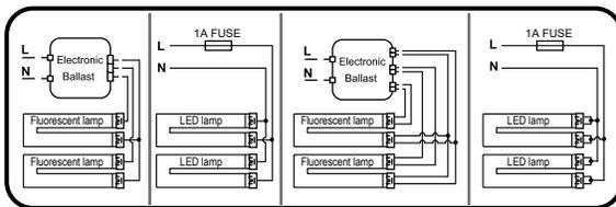
3) If two wires come from an existing lamp holder (rapid start type), these two wires should be wired or shunted together.
