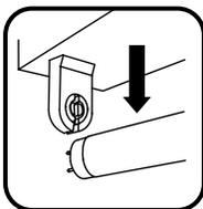
2) Remove all fluorescent lamps and ballast/wiring area cover. Cut the ballast lead wires about 6 inches away from each lamp holder.
