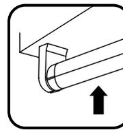
9) Adjust the color temperature switch on the lamp to achieve the desired performance. Install Type B double ended tubes.
