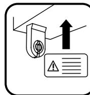
8) Install the retrofit kit Caution label in an easy to see location to ensure the user understands the system now uses LED Type B double ended tubes, and the use of fluorescent lamps may result in damage or injury.
