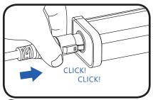
5 Insert the female connector of the batten jumper cable so that it fully engages the male connector of the luminaire currently being installed as indicated by hearing 2 clicks.
