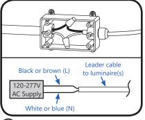
Inside the junction box, connect the line and neutral wires of the AC supply source to the line (black or brown) and neutral (white or blue) wires of the leader cable using suitable wire nuts. Install the junction box cover when complete.
