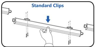
Unscrew the mounting clips to completely remove the batten.
