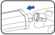
The Ensure that there is an end cap on the female connector on the last luminaire in the run.
