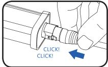
Remove end cap to the female connector where jumper cable will be installed. Insert the male connector of the batten jumper cable so that it fully engages the female connector of the **first luminaire** as indicated by hearing **2 clicks.**
