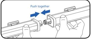
3 Slide the luminaire into the previous one in the run until the male connector of the luminaire fully engages the female connector of the previous one as indicated by hearing 2 distinct clicks. **Do not bend or otherwise exert excessive force on the luminaire connector.** Steps 3, 4 and 5 may be repeated for each additional luminaires in the run.
