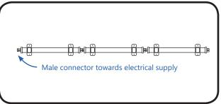
Place the luminaire on the surface with the male connector oriented towards the intended electrical supply. Install metal mounting clips over the luminaire, using two #10 (M5) self-tapping flathead screws to affix the metal mounting clips to the mounting surface.
