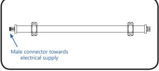
Place the luminaire on the surface with the male connector oriented towards the intended electrical supply. Install metal mounting clips over the luminaire, using two #10 (M5) self-tapping flathead screws to affix the metal mounting clips to the mounting surface.
