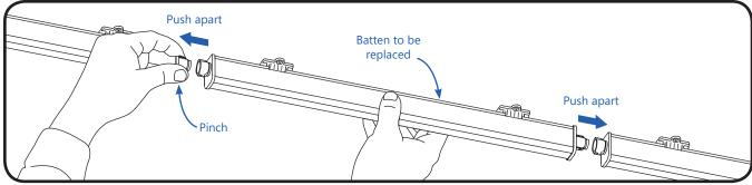
Unclip plugs on both sides of the batten to be replaced. Push apart battens on either side. **TIP:** Pinch the ends of the plug while pulling the receptacle end away.
