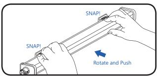
Press the luminaire into its mounting clips so that the male connector is oriented towards the intended electrical supply. *TIP*: Align luminaire on one side of the mounting clips; then rotate the luminaire until it snaps into other side of the mounting clips.
