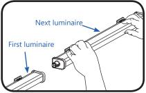
Press the next luminaire in the run into its mounting clips using the same procedure as Step 2.
