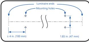
Pre-measure and mark each metal mounting clip screw location on the mounting surface. To avoid stress and damage to luminaire the entire mounting surface should be flat and the mounting clips be properly aligned. Refer to table on page 8 for required number of mounting clips per luminaire.
