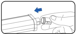
Ensure that there is an end cap on the female connector on the last luminaire in the run.
