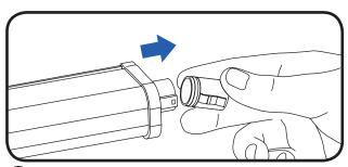
3 Remove the end cap from the female connector on the opposite side of the luminaire.
