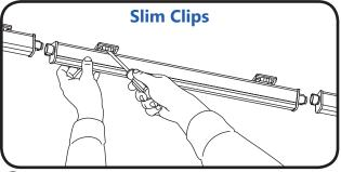
Using a screwdriver, gently pry the batten out of the mounting clips.
