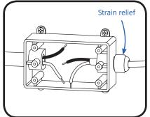
Insert the supply end of the leader cable through a suitable strain relief into a proper junction box for the location so that the leader cable outer jacket has passed through the strain relief. Tighten the strain relief onto the leader cable jacket.
