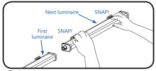
Press the next luminaire in the run into its mounting clips using the same procedure as Step 2.
