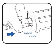
1 Insert the female connector of the batten leader cable so that it fully engages the male connector of the first luminaire in the run as indicated by hearing 2 clicks.
