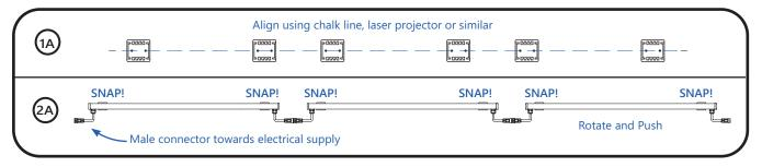
Parallel Layout NOTE: the recommended maximum space between parallel luminaires is 10" (245mm) for better optical uniformity.
