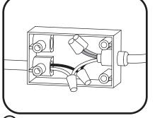
3 Inside the junction box, connect the line and neutral wires of the AC supply source to the line (black or brown) and neutral (white or blue) wires of the leader cable using suitable wire nuts. If 0-10V dimming will not be used, cap the dimming wires (purple and pink\*) with suitable wire nuts. Do not connect the dimming wires together or to line, neutral, or ground. If 0-10V dimming will be used, proceed to Step 4.
