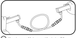
B Use a jumper cable to connect luminaires if the distance between them is too long.
