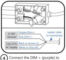
Connect the DIM + (purple) to the incoming dimmer circuit +. Connect the Dim – (pink\*) to the incoming dimmer circuit –.
