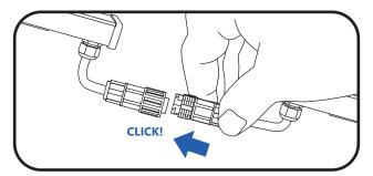
A Remove end cap from the female connector. Insert the male connector to the female connector. Make sure the connector is fully engaged as indicted by hearing a click.
