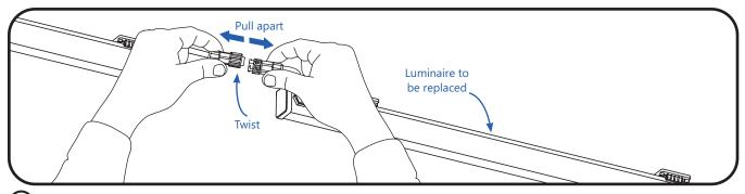
1) Disconnect the connector on both sides of the luminaire.
