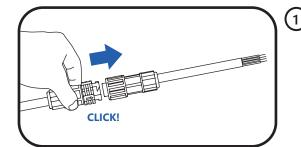
Insert the female connector of the leader cable so that it fully engages the male connector of the first luminaire in the run as indicated by hearing a click.
