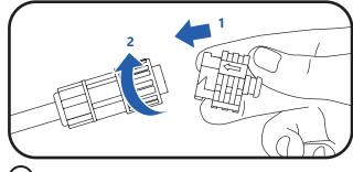
Insert an end cap into the female connector on the last luminaire in the run, and twist the end cap clockwise to secure.
