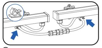
**Optional:** Secure the cables using the optional cable clamp accessory.
