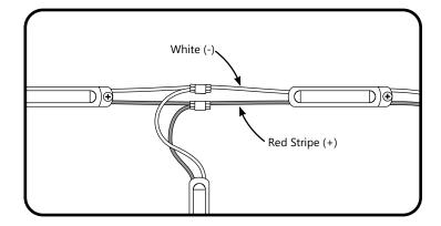
Connect LED strips using in-line (IDC) connectors or twist-on wire connectors appropriate for 18 AWG/0.82 mm2 wire.
