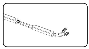
Must cap all exposed wires with appropriate wire connectors.
