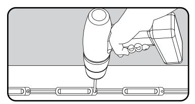
Use screws to secure the LED strip (minimum 1 self-tapping screw per foot/0.3m).
