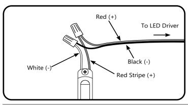
Connect the red stripe wire (+) of the LED strip to the red wire (+) of the LED Driver. Connect the white wire (-) of the LED strip to the black wire (-) of the LED Driver.
