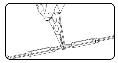
Measure and cut LED strip to the appropriate length. Cuts can be made between any of the modules.
