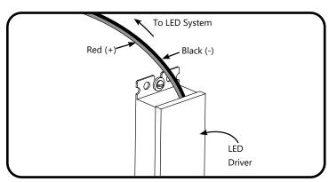
Run a wire from the LED Driver to the first LED module on the strip.
