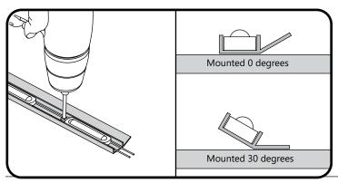
**Optional:** LED strip can be snapped into track and fastened with self-tapping screws.
