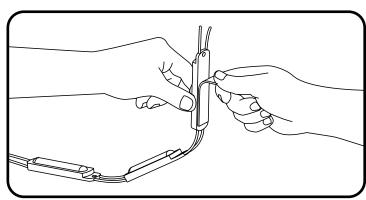
Remove tape backing and stick LED modules into place. Continue until you have reached the end of the strip.
