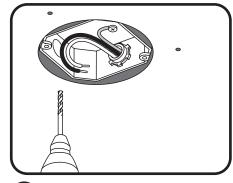
Mark ceiling around electrical box and drill 3 holes.
