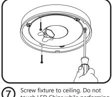
Screw fixture to ceiling. Do not touch LED Chips while performing this step.
