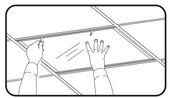
1 Rotate latches to unlock the front bezel.
