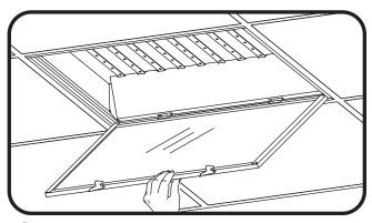
Swing down panel and lift off front bezel with diffuser
