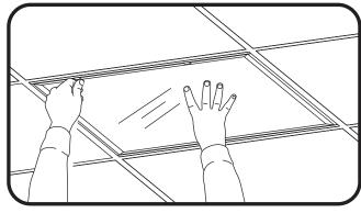
Hang panel on its hinges and swing up into place. Rotate latches on front bezel to fasten it.
