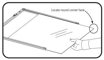
Remove the old diffuser by sliding it toward the side without end rail. Insert new diffuser, keeping the round corner of diffuser on bottom right.
