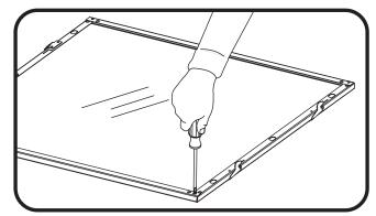
5 Reattach end rail with screws.
