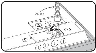
Install listed electrical fittings in the knockout holes for wire protection. Connect the AC line to the luminaire internal wires according to the wiring diagrams using 18-14AWG twist-on wire connectors.
