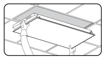
Install the unit into the reserved hole in the ceiling.
