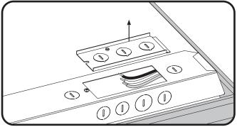
Remove electrical enclosure cover. Remove knockout for AC line input wires.
