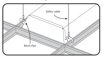
Bend the 4 clips to secure the luminaire in place. Install the safety cables through the holes on the clips (per local building codes, safety cables by others).
