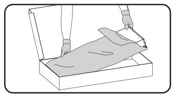
Carefully unpack unit from its packaging. Properly inspect for defects before installing. Wear work gloves to prevent dirt and oil from being transferred to the luminaire.
