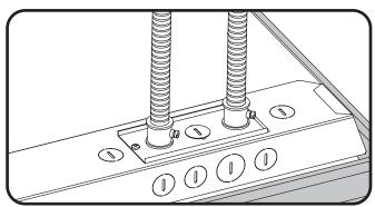
Replace electrical enclosure cover and secure it with the screw
