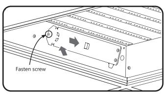
Push plate into opening and shift to the right. Fasten screw of driver plate to the housing.
