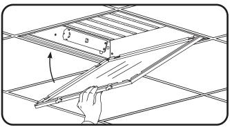
Hang panel on its hinges and swing up into place.
