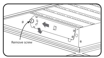
Unfasten screw holding driver plate. Grab tab and shift plate to the left and pull outward.
