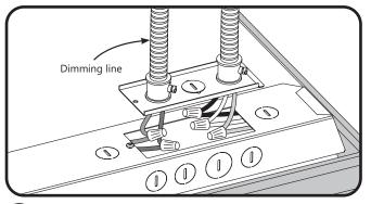
Install listed electrical fittings in the knockout holes for wire protection. Connect the dimming control (grey/pink and purple) wires of the LED driver using 18-14AWG twist-on wire connectors.
