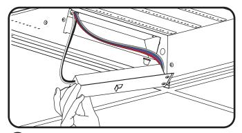
Remove driver plate. Driver is attached to cover plate and wiring is accessible when cover plate is removed. Connect the AC line to the luminaire internal wires according to the wiring diagrams using 18-14AWG twist-on wire connectors. Connect the dimming control (pink and purple) wires of the LED driver using 18-14AWG twist-on wire connectors.Install listed electrical fittings in the knockout holes for wire protection as well as lead wires into the electrical cavity.
