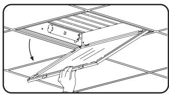
Swing down panel and lift off front bezel.
