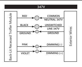
NOTE: Dimming leads for the VQ and V1 catlogic option are 0-10V dimming, grey/pink (-), violet (+). Dimming leads for the LE option are Lutron Ecosystem - pink is E1 (-), violet is E2 (+). Assent, LBT & LBR Installation Guide
